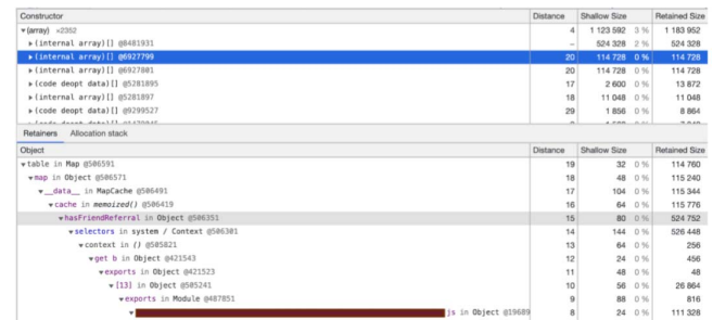
Fig. 4. Memory leak detection in fiit website using heap snapshots.
